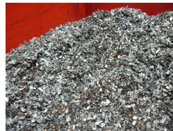
Delaminated fraction LFP 3,09 kg
