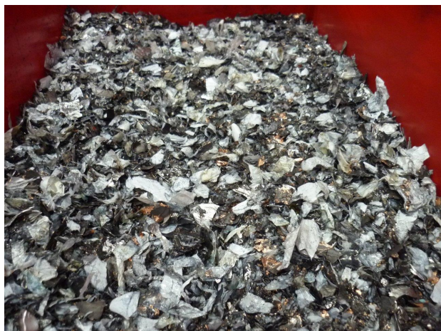
Initial fraction LFP 3,15 kg
